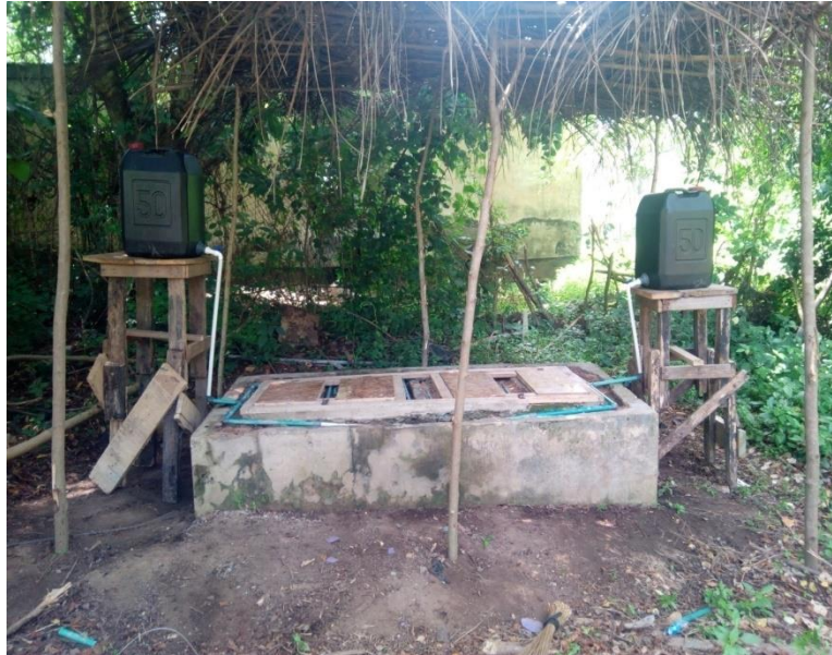
Plate 1: Evaporative Cooling Chamber With Water Reservoir.
